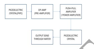
When the mechanical vibrations reach the receiver section, they are received by a piezoelectric crystal which again converts mechanical vibrations into electrical signals. These signals are again amplified using OP-AMP IC 741. Then the output of OP-AMP is passed to a microcontroller Atmega 16. The microcontroller interfaces the received output to a 4x1 inches LCD. The LCD displays the digital output.
