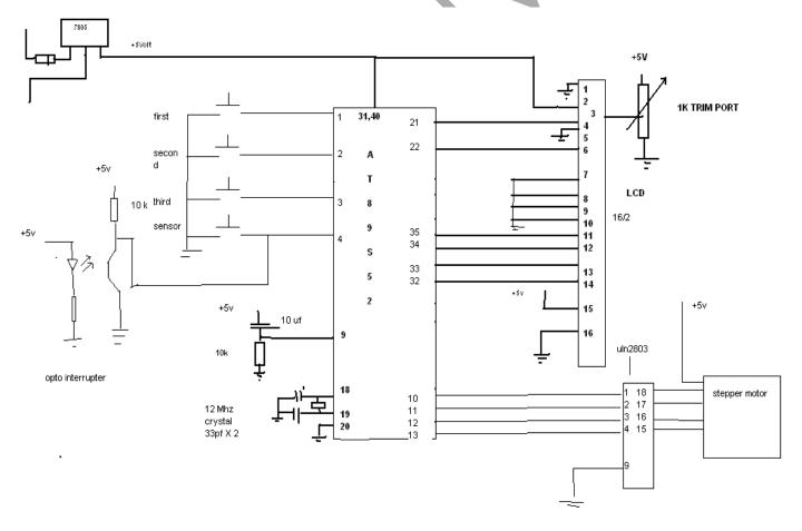
This project consists of two IR receivers and transmitter pair that control the automatic gates and vehicle detection as it passes through it. An LCD displaying the exact number of cars parked in the bay and possible
